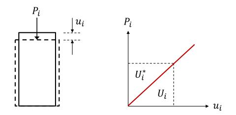
As previously defined, the general expression for strain energy, shown as the area under the load-displacement plot above, is:.
